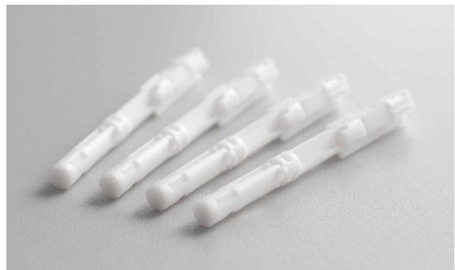
Injection molded in a 4-cavity mold, the delicate lancet holder is made from teflon-modified polyoxymethylene (POM) and part of a lancing device with mechanical functions, openings and operating elements
