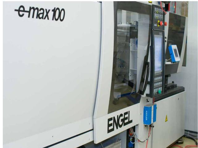
A Kistler CoMo Injection Type 2869B2... (on the right, beside the injection molding machine) is monitoring the production of plug connectors
