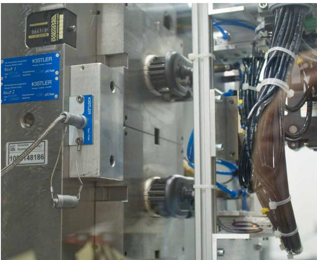
The multi-channel plug connector located on the mold exterior integrates all signals in one cable and connects to the CoMo Injection system
