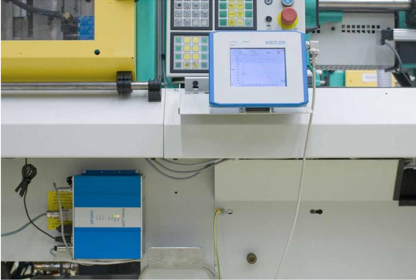
The CoMo Injection process monitoring system (below) with display screen (on the right, beside the operating panel) controls the reject gate for free-falling components at the front of the injection molding machine
