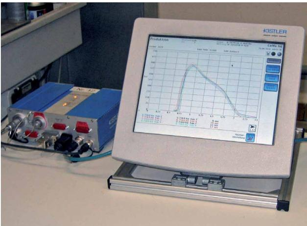
The monitor displays the cavity pressure profile of an 8-cavity mold
