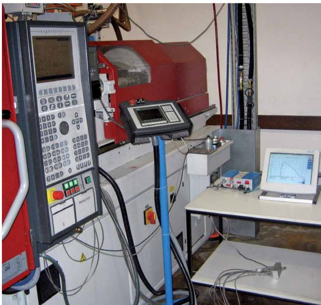
A Kistler CoMo Injection process monitoring system Type 2869 (on the right, beside the injection molding machine) monitors the production of plug connectors
