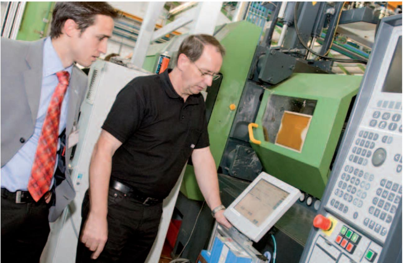
At HEWI, CoMo Injection process monitoring systems are mounted on mobile carriages. This way, they can be moved from machine to machine
